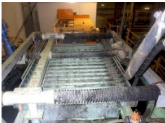
Figure 7: Electrowinning cell (foreground) and rectifier (background) in full production at the Intec Copper Process demonstration plant.
