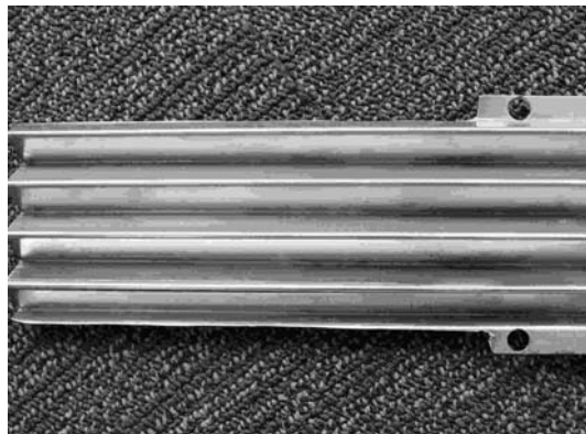
Figure 3 – Laboratory-Scale Corrugated Titanium Cathode
