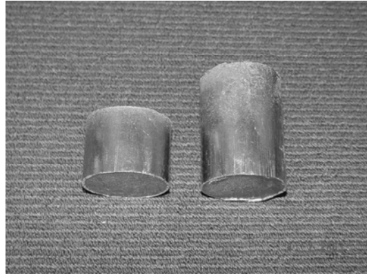
Figure 19 - Two-stage Ram-Pressed Briquettes
