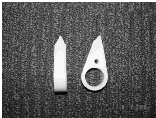
Figure 13 - Wiper Teeth Design for Revised Wiper Bar
