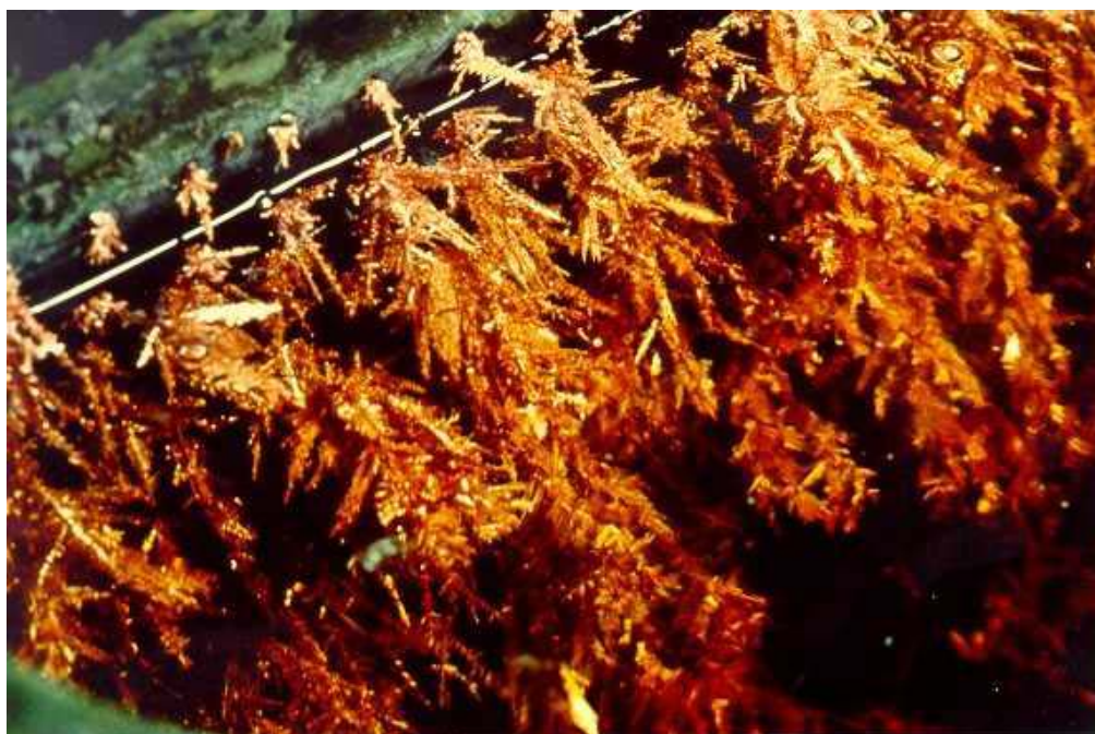
Figure 6: Copper dendrites growing on the cathode.
