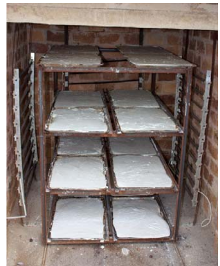
Figure 2: High-grade calcium sulphate product samples drying in the oven at the Liuzhou project pilot plant
