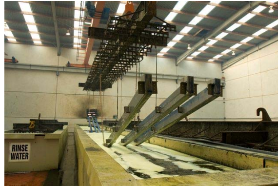
Figure 1: A galvanising industry acid 'pickle' bath
