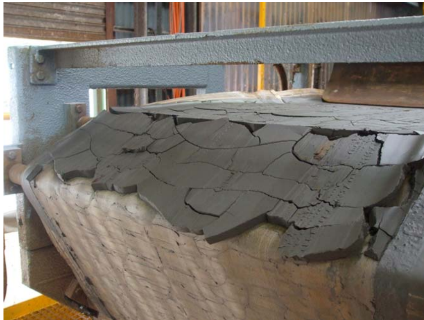
Figure 7: The clean, homogenous heavy metal sulphide filter cake shown during recent trials at Intec's Burnie Demonstration Plant
