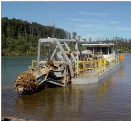
▲ The dredge at work on the Hellyer tailings dam.
