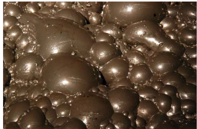
Above – Bulk zinc concentrate being recovered in the froth flotation circuit at the Intec Hellyer Mill
