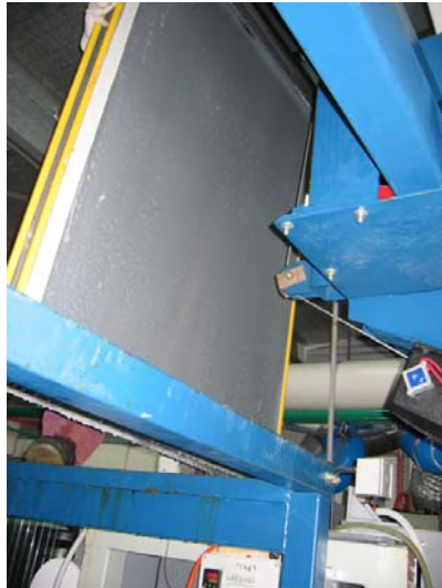
Figure 2: Two jumbo-sized cathodes being hauled above the electrowinning cell at the University of Sydney, having been plated at 400 amps/m 2 to produce 100kg of Special High Grade (99.99% pure) zinc per day.
