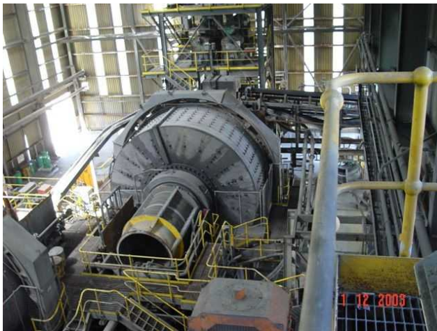
Figure 4: 2MW SAG Mill at Hellyer
