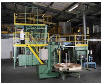
Figure 10: Intec copper product being cast into 8mm oxygen-free copper rod at Rautomead's test facility
