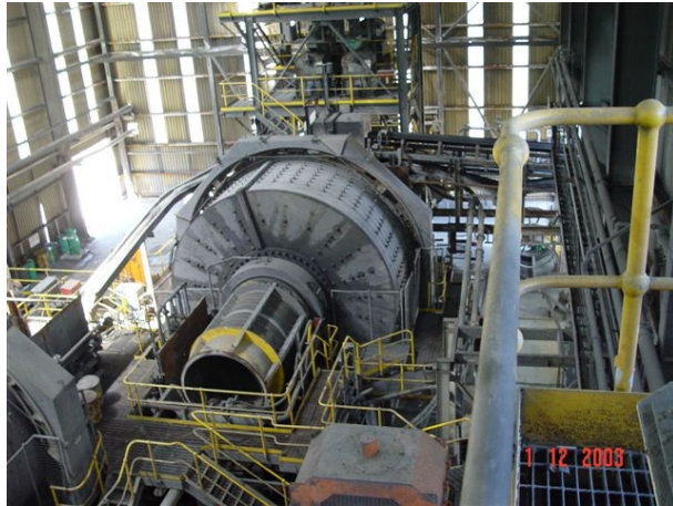
Figure 4 The 1.5mtpa SAG mill at Hellyer
